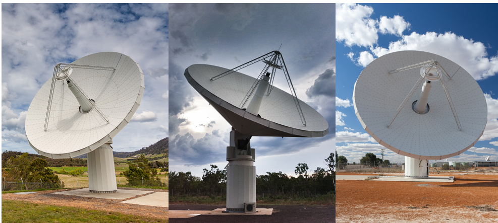
Figure 2: The three 12-m diameter telescopes of the AuScope VLBI array. From left to right: Hobart, Katherine and Yarragadee.
